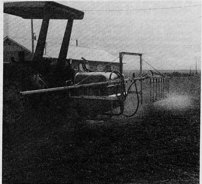
Fig. 1. Commercial spray boom with half of the boom rigged with 46-cm drop tubes.
